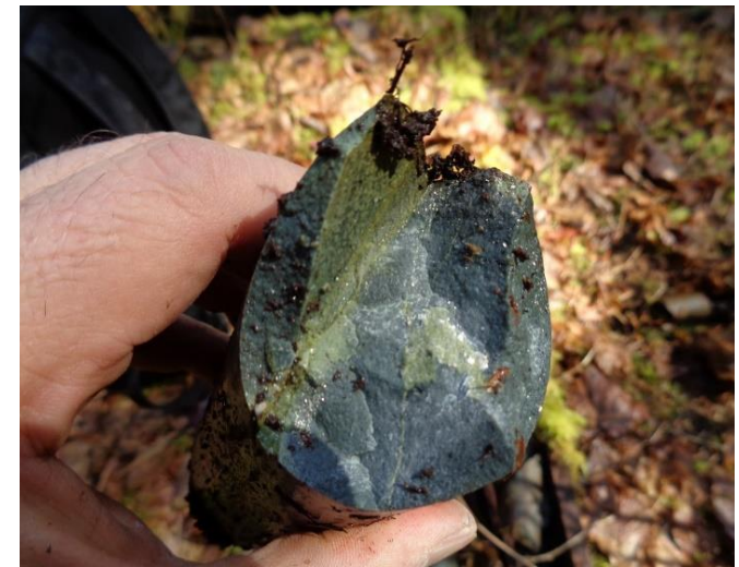
Drill core fragment showing fine disseminated pyrite with chlorite and epidote, typical of propylitic alteration.
