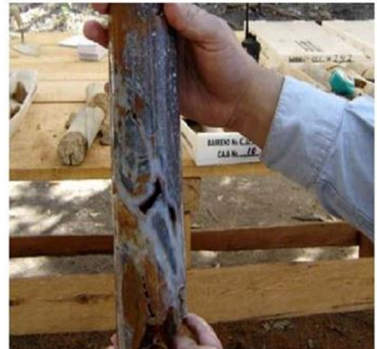
Drill core from Cerro Di Oro zone showing quartz stockwork.
