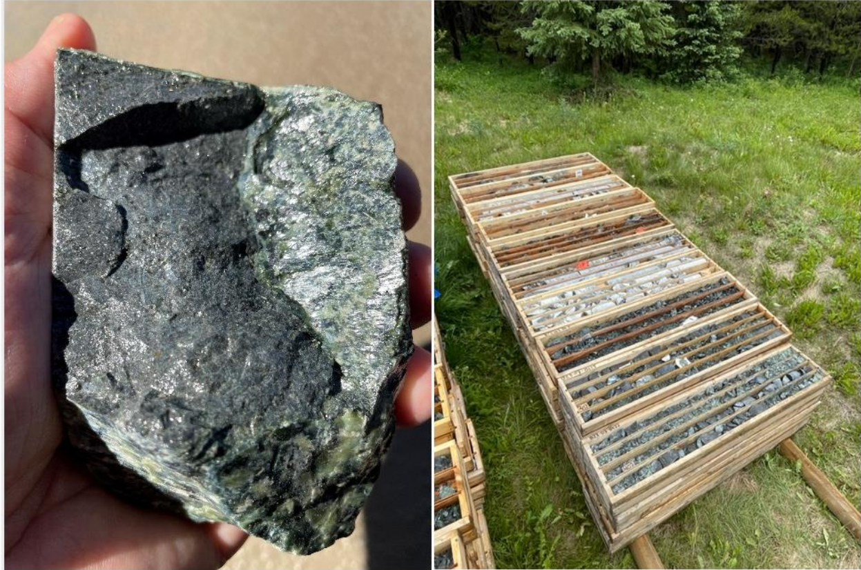
Figure 3. Left: core sample from drill hole B23-01 showing rich magnesium and nickel mineralization in black and serpentine in green. Right: Drill core from hole B23-03 in core sample boxes at storage facility.
